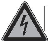
Risk of electric shock which could cause personal injury or material damage. Always switch off the power supply before carrying out any work.
