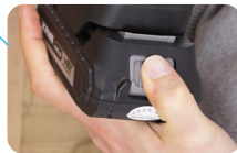
BATTERY EJECT BUTTON
